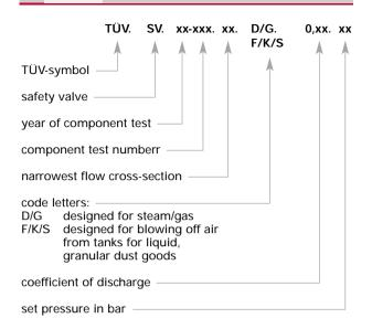
We check the safety valves for pressure resistance and tightness, adjust the requested set pressure and seal them.
