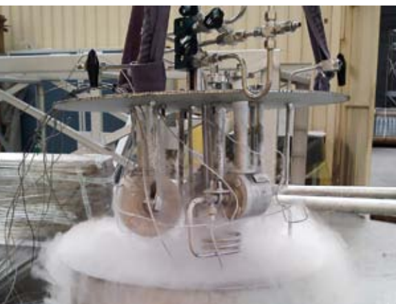
Leakage test at very low temperature
